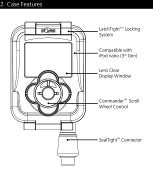
IMPORTANT: Make sure the seal is fully seated against the housing base each time you close the housing. Use the lid to compress the seal into the base if required.
